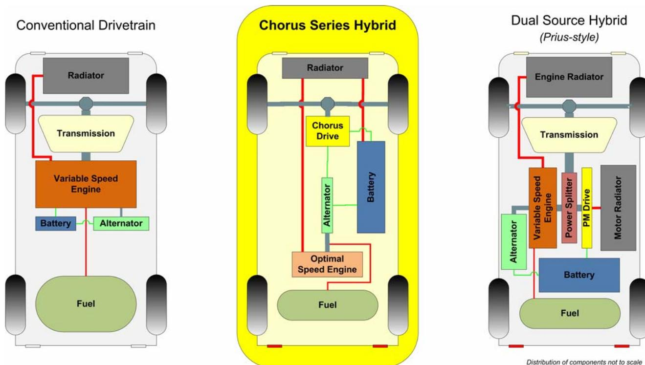
Chorus has been exploring simple series and parallel hybrid approaches, in an attempt to simplify the entire system. We believe that the series hybrid approach offers the opportunity to significantly improve efficiency while keeping the system simple. This will reduce costs, and still provide the required performance.
